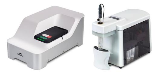
The Malvern Zetasizer Ultra Red system is provided with a He-Ne 632.8 nm laser with a constant power of 10 mW and an avalanche photodiode. The system allows to measure the size and zeta potential of particles, alongside their concentration. Using the MADLS system, the hydrodynamic diameter and concentration of particles can be determined in the range from 0.3 nm to 15  $\mu$ m and 10<sup>8</sup> to 10<sup>12</sup> particles per mL, respectively.
