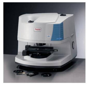
Nicolet<sup>TM</sup> iN10 MX microscope is designed for imaging in mid-IR range. It is equipped with ceramic IR source and three detectors: DTGS, MCT-A and an array of 16 MCT-A detectors. The equipment allows registration of absorption spectra in the wavenumber range of 600-4000 cm<sup>-1</sup>. Chemical mapping can be performed with the spatial resolution of 25x25  $\mu$ m<sup>2</sup>, or using special conditions even 6.25x6.25  $\mu$ m<sup>2</sup>.
